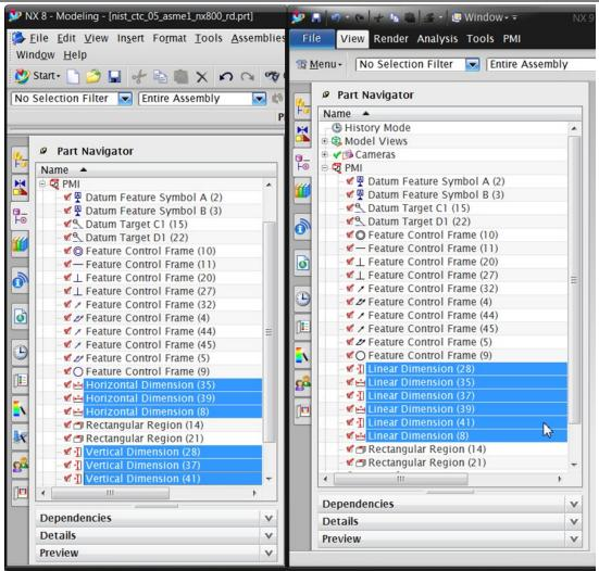
Figure 6: NX 8 vs. NX 9 Dimension Display Names
