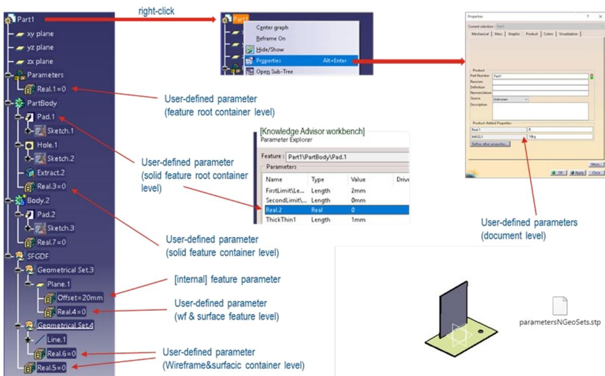
Figure 12: Overview on Parameters and Properties defined in the CATIA model
